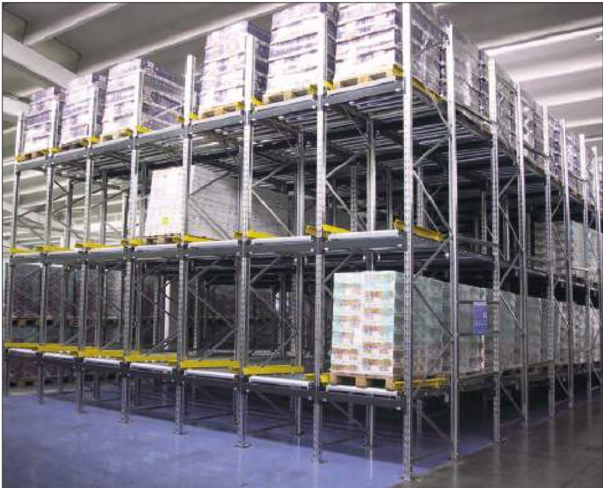
Magazzino dinamico FIFO a tunnel singolo / FIFO dynamic warehouse with single tunnel
